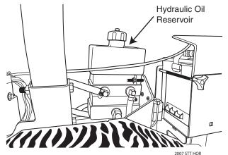
Figure 7-2. Hydraulic Oil Reservoir
